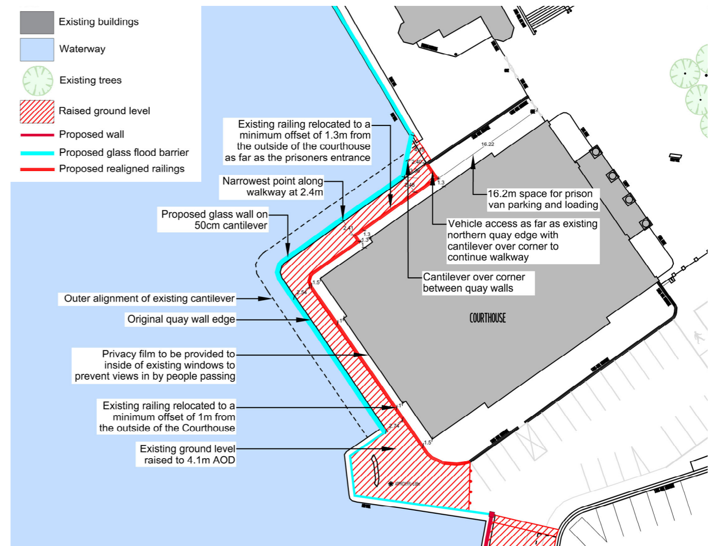
Design Proposal: Realigned Courthouse railing with reduced size of cantilever.
